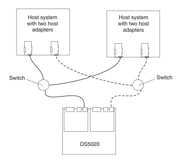
Figure 58. Example of a dual SAN fabric configuration
